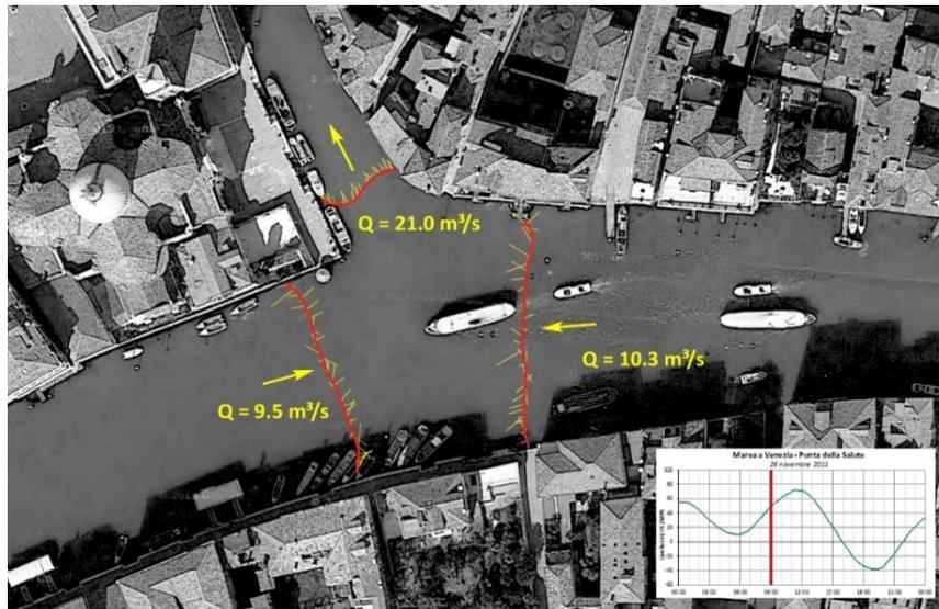
Fig. 10 – Current measurements at the intersection of the C. Grande – C. Cannaregio carried out on 26/11/2011 during the incoming tide (between 8.57am and 9.06am). In the three sections, measurements are not simultaneous therefore the continuity is not rigorously respected (data supplied by ing. P. Peretti).
