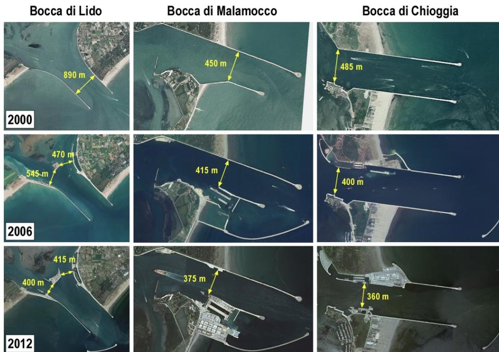
Fig. 1 – Narrowing of the inlets due to construction of Mo.S.E. (geo-referenced aerial photos from the *GeoPortale Nazionale* of the Environment Ministry <http://www.pcn.minambiente.it/GN/>)
