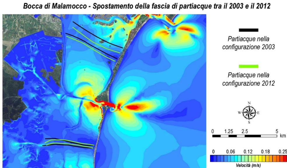
Fig. 9 – Displacement of the “watershed strips” marking the Malamocco sub-basin, obtained using the hydrodynamic model. The black lines show the “watershed strips” determined by the previous configuration, pre Mo.S.E. structural works (2003) and the green lines mark the “watershed strip” determined using the post-interventions configuration (2012).
