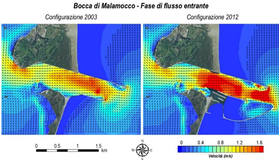
Fig. 8 – Comparison between velocity fields with the incoming tide calculated with the 2D model, considering two configurations: 2003 e 2012.
